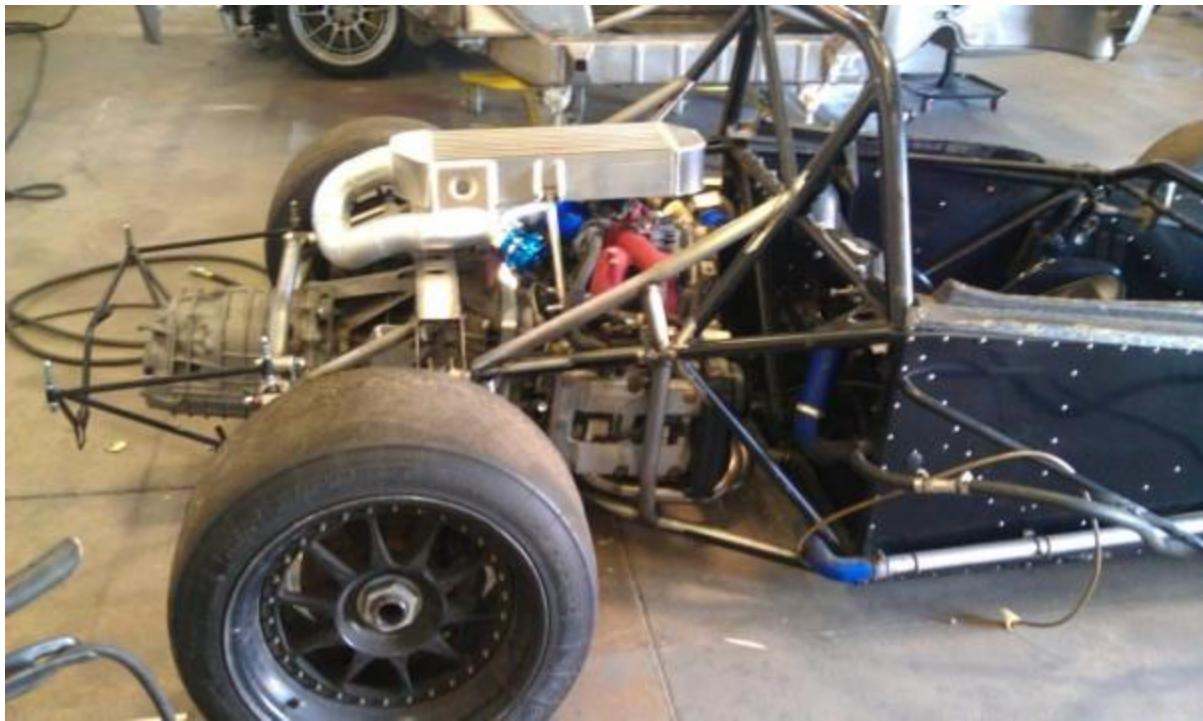
Here is a close up of the “engine bay”. The gold foil is heat protection for the chassis as well as the passenger compartment and the body. Everything in this car is a super tight fit with little room to spare.
