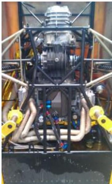
Here is an under body shot looking up. You can see the Cosworth dry sump setup, hand built headers, and the gold foil on the chassis to keep the passenger compartment temps down. On the other side of the gold foil is the gas tank which also happens to be the back of the seats.
