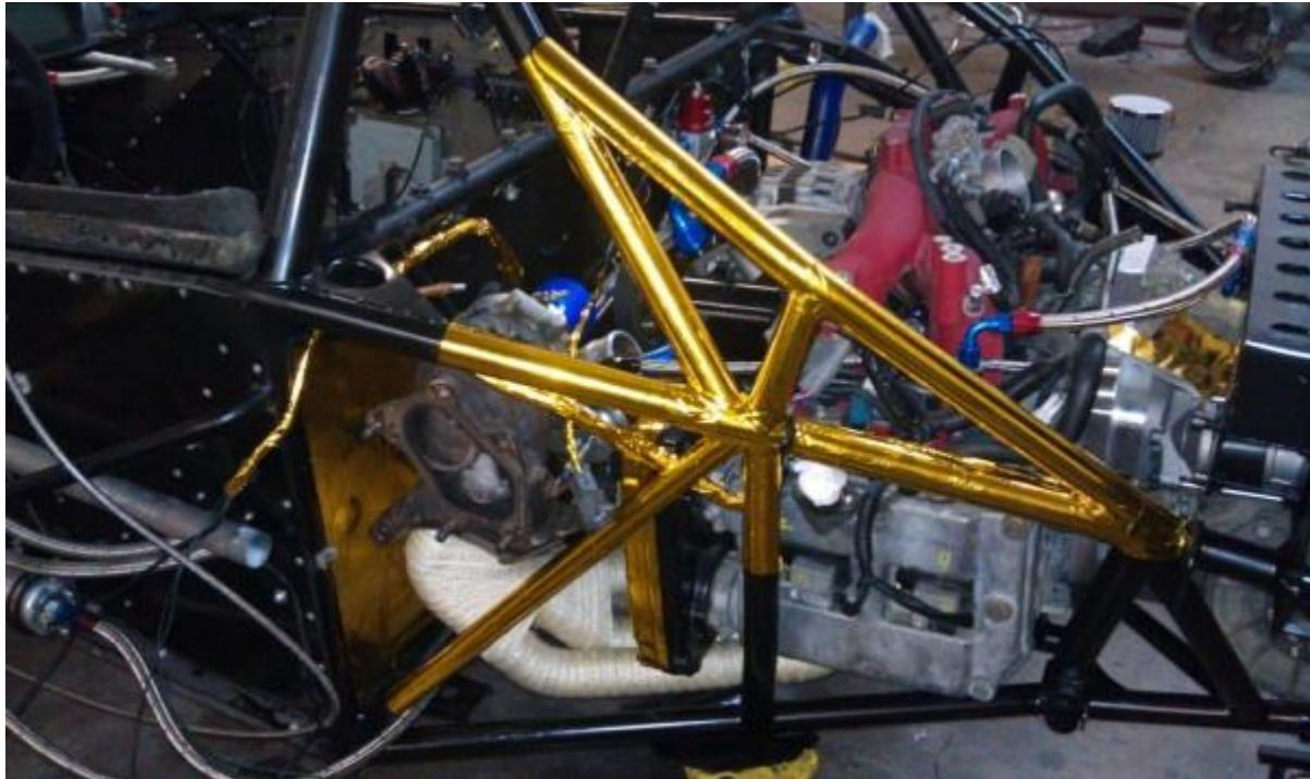
Here you can see the exhaust and intercooler installed.
