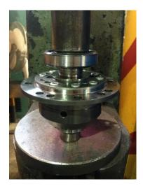
29. Reassemble the Main Shaft with the new bearings and forward gear. Unless the gearbox has sustained substantial damage, reverse gear is commonly used again.
