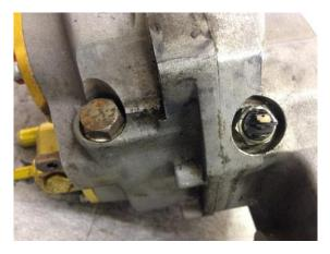
9. Remove Index Plunger/Detent, TQ0130 using a machined down 19mm long 3/8 drive socket.
