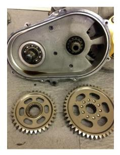
7. Remove TQ0036 Input Shaft Coupling, this will be replaced.
