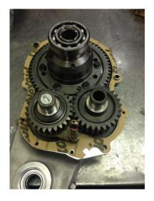
32. When refitting Differential Bearing Retainer (TQ0127), Oil pump (TQ0025) and Breather (TQ0120); ensure to use silicone sealant as the joining compound as demonstrated in step 27.
