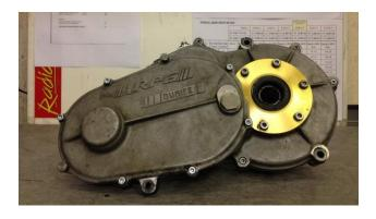
2.Remove 6x M6x16 cap head bolts (TQ0143 schnorr type M6 washer) along with 2x 13mm threaded stud (TQ0121).
