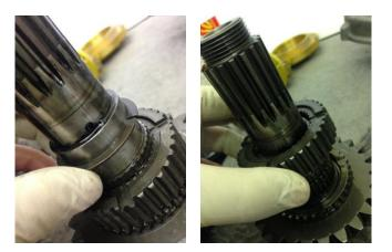
23. Inspect needle roller bearings TQ0138 and TQ0135for pitting, over heating or any other wear marks.Replace if necessary.
