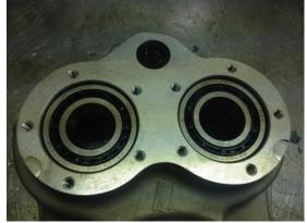
27. Take the Front Casing (TQ0112) and Differential Bearing Retainer (TQ0118); apply a small amount of silicone sealant around the inner edge of the Bearing Retainer (TQ0118) and fit it to the Front case and tighten evenly 5x M8x25 to 35NM /25Ft.lbs. Wipe the excess sealant away and turn the Front Casing over.
