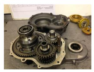
17. Remove TQ0137 bearings using a nylon drift and nylon hammer.
