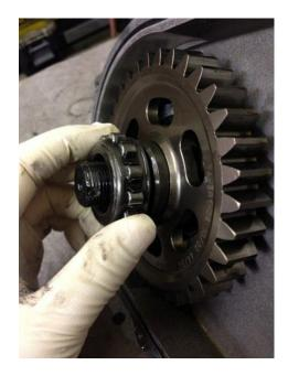
5. Remove TQ0073 Input Spacer, tapered side facing bearing.
