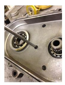
15. Using a nylon hammer break the seal of the two casing.
