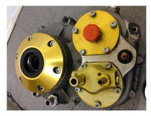
11. Using a flat head screwdriver pry the oil pump and breather cover from the casing using the machined grooves.
