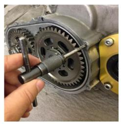
3.1 Remove TQ0037, Locknut Main Shaft (left-hand thread) using a 42mm impact socket.
