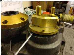
12.1 Remove 6x M8x16 cap head screws for TQ0127 differential retaining plate and remove plate using two screwdrivers to pry the plate from the casing.
