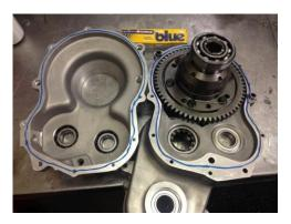
31. Take the Rear Case (TQ0111); ensure that Bearings TQ0136 are fitted along with Oil Seal TQ0057. Apply Hylomar Universal Blue Gasket and Joining Compound around the Rear Case (TQ0111) and join the two cases together ensuring to locate the two hollow Dowels (TQ0132), before tightening.
