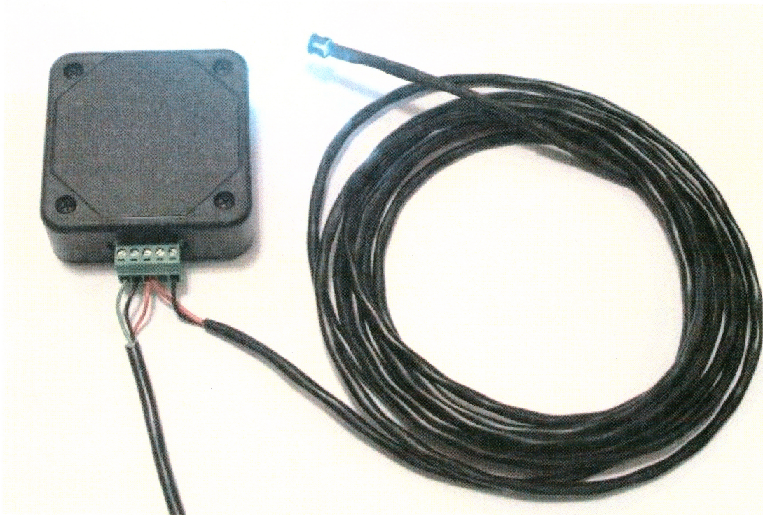
Typical Wiring Application with Single LED
