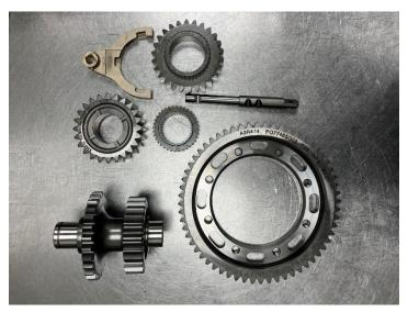
When fitting TQ0731 rebuild kit, all provided parts must be fitted as they are not backwards compatible with the old internals. Customers are advised to upgrade their GDU at the point of a normal GDU rebuild.
