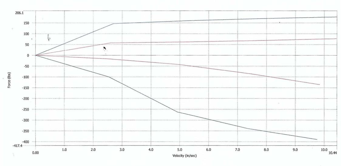
RAD 1-2 DAMPER TESTED AT 2.5 5 7.5 10IN/SEC 2` STROKE UNIT TESTED AT MIN & MAX 23/10/2018
